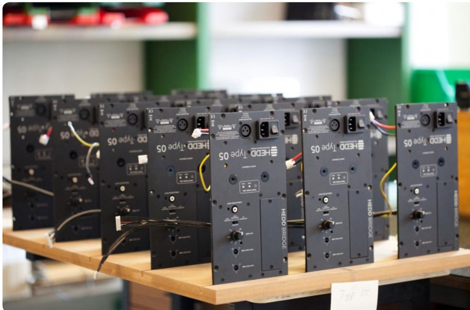
On the rear panel, in addition to the volume control, there are switches for selecting the source among balanced XLR, unbalanced RCA and HEDD BRIDGE, and recessed trims for high (shelving + / 4 dB @ 20kHz) and low (shelving + / 4dB @ 50Hz).
