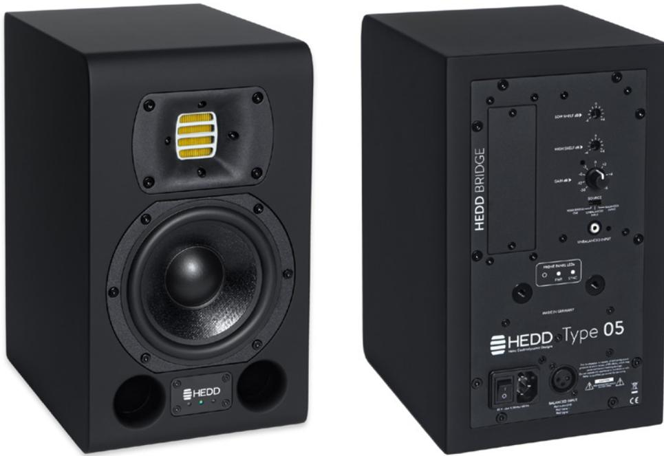
Type 05 is a fairly compact monitor (L = 180, P 228, H 308mm.) equipped with a 152mm woofer. (6" not 5", as one might argue from the name!) in very stiff composite honeycomb while the ribbon tweeter adopts AMT technology for a 506mmq emission area, equivalent to a 2" dome tweeter but without having the side-effects of such component at higher frequencies.
